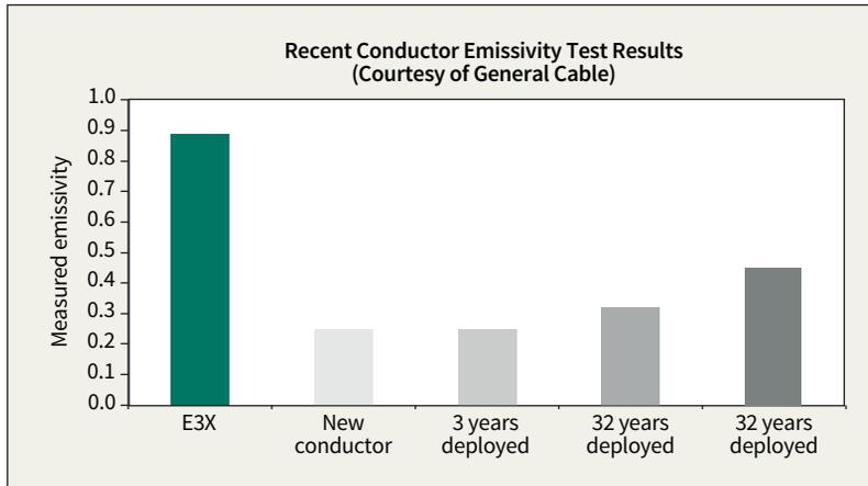
E3X Technology can be applied to increase capacity of any aluminum conductor deployed by Avista.
