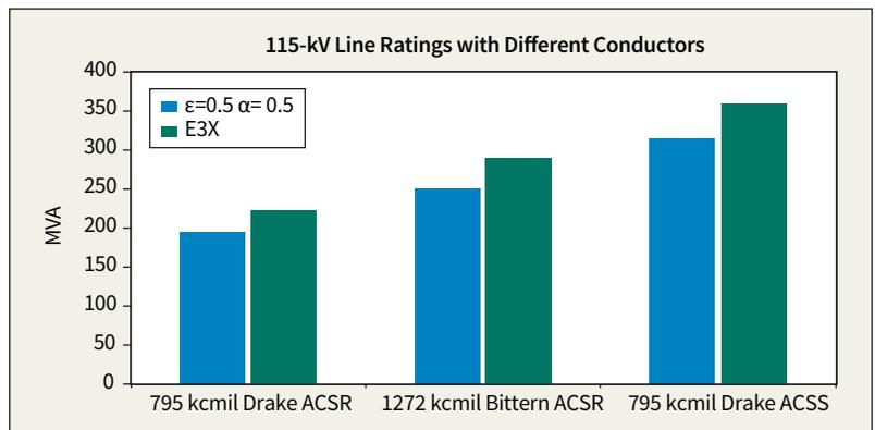
Selecting line-rating values can be highly subjective without engineered emissivity from E3X Technology.
