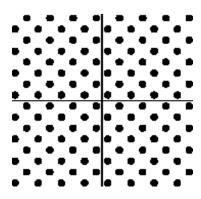
Tomlinson-Harashima Precoded (THP) 16 discrete levels: 2-dimensional latticed pattern 16 voltage levels coupled w/ 16 time intervals on each pair
