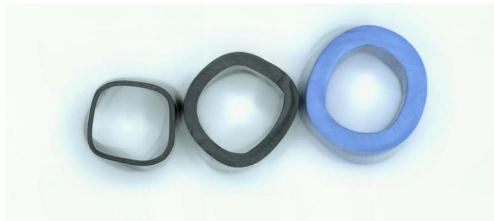
Figure 3: (Left to Right) Cross-sections of a standard premise cable jacket, an AWM 600V jacket, and an AWM 600V PLTC jacket.
