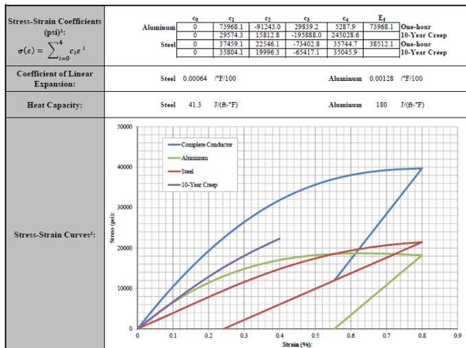
\* Stress-Strain Coefficients and the Final Modulus are in units of psi/100. The values provided may be directly inserted into a PLS-CADD conductor ".wu" file using the US units format.
